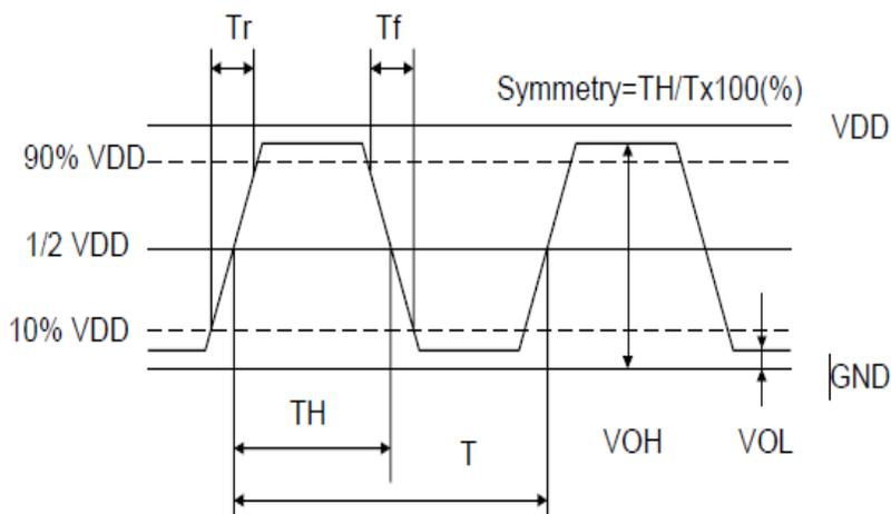
Waveform measurement system should have a min. bandwidth of 5 times the frequency being tested.
