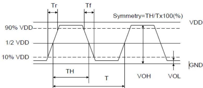
Waveform measurement system should have a min. bandwidth of 5 times the frequency being tested.
